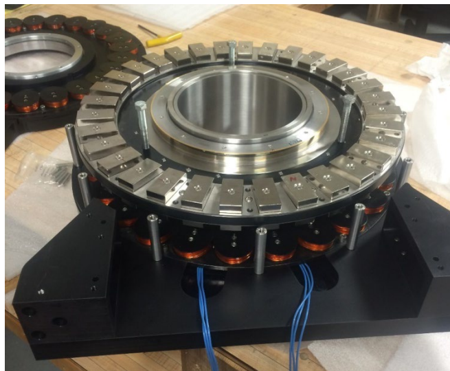
A direct-drive motor assembly showing the array of magnets and coils.
