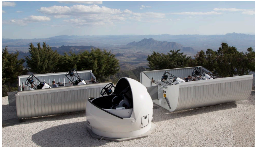
MINERVA, the Miniature Exoplanet Radial Velocity Array, located on Mt. Hopkins in Arizona, consists of four 0.7-m PlaneWave Instruments CDK-700 telescopes housed in two flip-open enclosures. An optical fiber from each telescope are combined to feed a spectrograph with an equivalent single-telescope aperture of 1.4-m. Alternatively, the four telescopes can be operated independently when cameras are selected instead of the optical fiber feeds. The fifth CDK-700 in the dome is not part of the four-telescope array.
