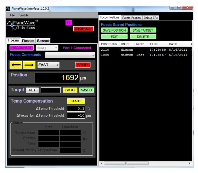
At the top of the window there are three tabs, Focus Position, Rotate Position, and Debug. The Focus Position Tab shows the saved focus positions and the Rotate Position Tab shows the saved rotator
