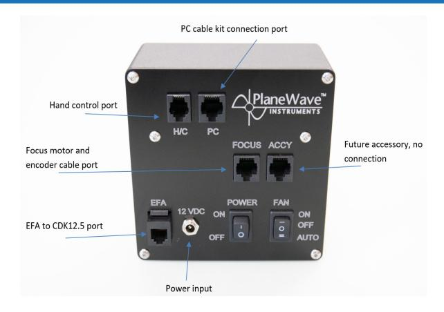
Note that the 12VDC power is attached to the EFA control electronics rather than to the rear of the telescope. Fan control and power are provided via the RJ12 6P6C modular cable from the EFA port to the rear panel of the telescope depending on switch position selection.
