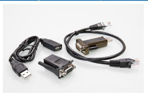
While the RJ45 "PC" port on the EFA is the similar to that used for Ethernet, the protocol used for communication with the PC is serial/RS232 and the wiring differs from that of Ethernet. The included USB-to-serial adapter, USB extension cable, DE9-to-RJ45 and standard CAT5 cable must be used rather than a direct connection via Ethernet to the PC. If needed, a longer CAT5 cable can be used to extend the connection between the DE9-to-RJ45 adapter at the PC and the EFA.
