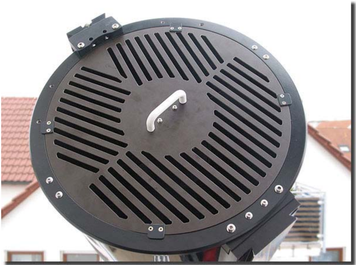
Animation of diffraction effects while focusing with a Bahtinov-mask
